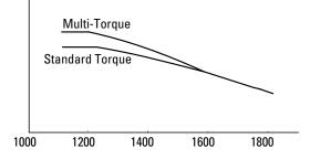
The ECM determines when the vehicle is in the top gears by calculating the ratio of engine speed to vehicle speed. The number of affected gears is determined by the selected Multi-Torque Rating feature.
