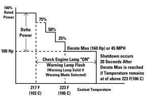
As Coolant temperature rises to 217 °F (103 °C) the engine is derated by 25% of the Delta Hp. In this example 240 Hp x .25 = 60 Hp. The driver would have 340 Hp available. If the driver reacted by downshifting, for example, and the temperature did not rise, the power would stay at this level.
