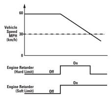
Engine Retarder Minimum Vehicle Speed is similar to Low Cruise Control Speed Set Limit. Engine Retarder Minimum Vehicle Speed sets the minimum vehicle speed at which retarder operation is allowed. This parameter affects both the Engine Retarder Solenoids and any auxiliary brake. Setting the Engine Retarder Minimum Vehicle Speed to 0 (Zero) disables this feature.
