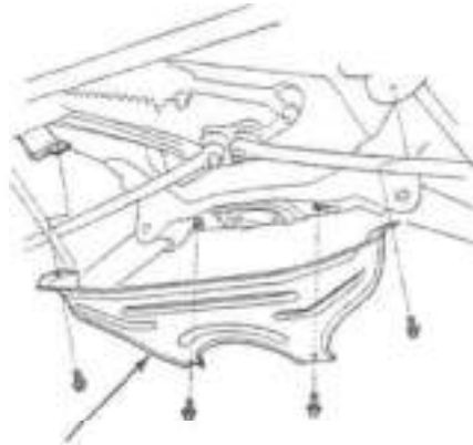
Front Air Duct
